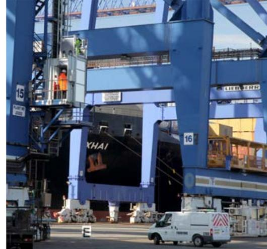
STROS rack and pinion industrial elevators are primarily used as a means of vertical access for personnel and material in various industrial facilities. They are designed to reliably perform with long life cycles in harsh environments. They are built to comply with the European Machinery Directive, or they can meet the ASME A17.1/B44 code enforced mainly in the US and Canada.
