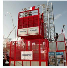
Among other applications, construction hoists are typically used on construction sites with high requirements for the transport of people and materials, in the construction of high-rise buildings and bridge pylons. STROS hoists are designed and manufactured for long life and reliability. This hoist is designed for operation on two masts.
